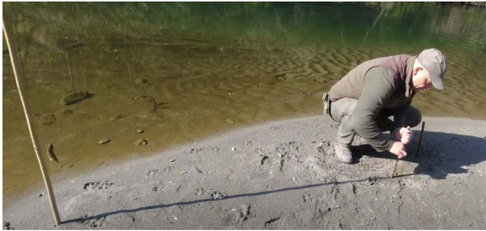
Figure 5: Wait about 15 minutes for the shadow to move. After 15 minutes have elapsed, mark the location of the tip of the shadow with another small stick.
