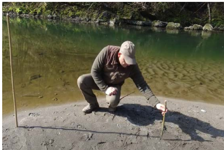
Figure 4: Place a small stick on the tip of the shadow of the first stick.
