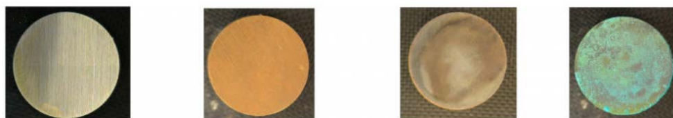
Image 5: Various patinations for studies in a laboratory environment https://www.alternator.science/sl/daljse/kako-se-stara-bron-lepota-staranja/
